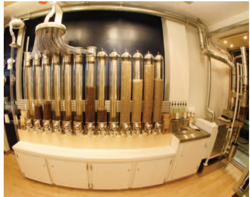
The Roasting Plant's pneumatic bean system. Courtesy of Roasting Plant Coffee, New York City.
